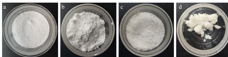
a-770FCP b-挥发油-770FCP (1:5) c-挥发油-770FCP (2:5) d-挥发油-770FCP (3:5) a-770FCP b-volatile oil-770FCP (1:5) c-volatile oil-770FCP (2:5) d-volatile oil-770FCP (3:5)
