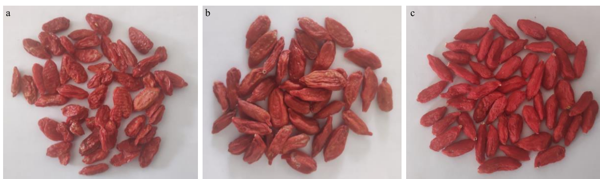
a-自然晾晒 b-远红外真空干燥 c-超声+远红外真空干燥 a-air drying b-far infrared vacuum drying c-ultrasound + far infrared vacuum drying
