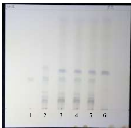
1-黄芩苷对照品 2-黄芩对照药材 3~5-补肺颗粒供试品 (批号 001、002、003) 6-缺黄芩阴性样品 1-baicalin reference substance 2- Scutellariae Radix reference material 3-5-BuFei Granules (Batch No. 001, No. 002, No. 003) 6-negative sample without Scutellariae Radix
