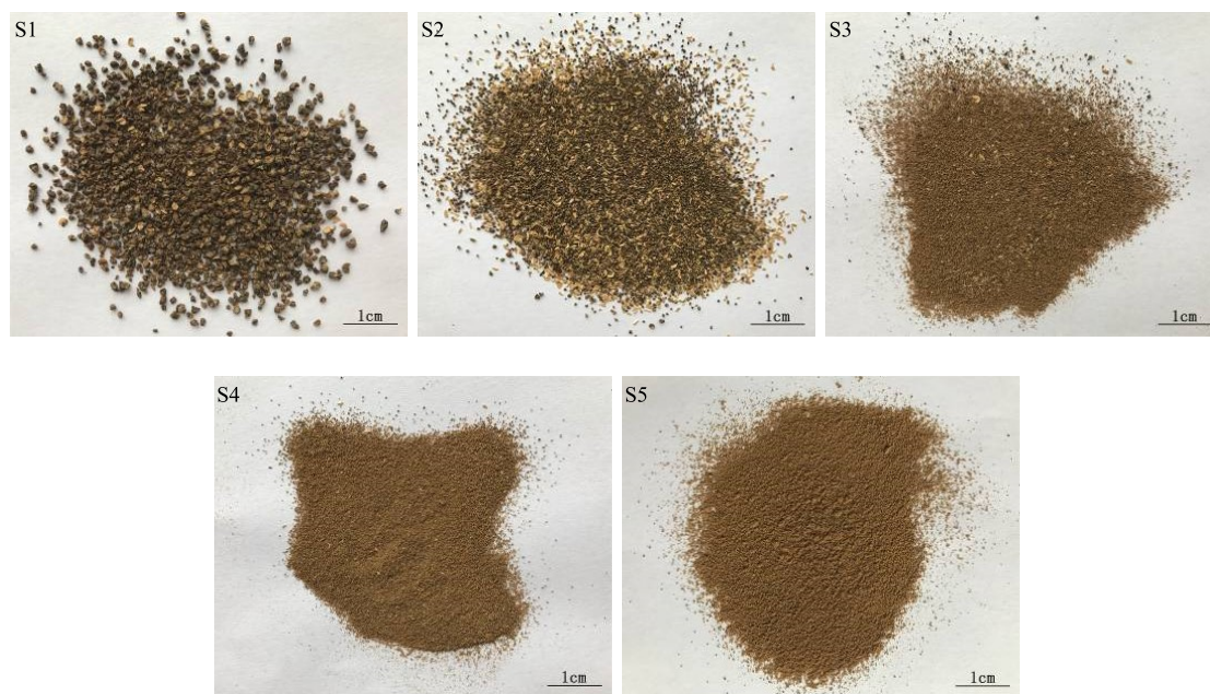
S1-研钵研碎, 不过筛的粉末 S2-过不了 3 号筛的粉末 S3-不过筛的全粉 S4-过 3 号筛的粉末 S5-过 5 号筛的粉末 S1-powder grinded with a mortar, but not sieved S2-powder can't pass 3 # sieve S3-whole powder not sieved S4-powder can pass 3 # sieve S5-powder can pass 5 # sieve
