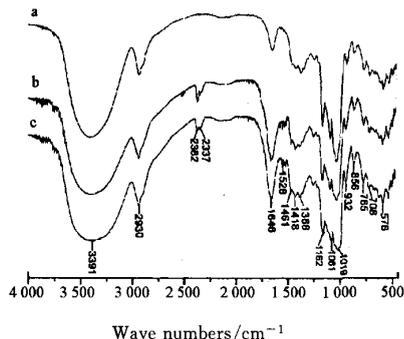
Fig. 2 FT-IR spectra of two powders of *Fritillaria L.* and potato starch
