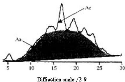
Fig. 1 Calculation of relative crystallinity degree
