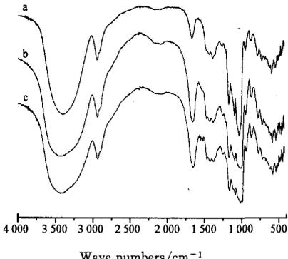
Fig. 3 FT-IR spectra of potato starch and two powders of *Fritillaria L.* extracted with 85% ethanol at 45 °C for 48 h
