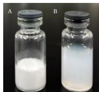
图 5 Gal-Art-NVs 冻干粉 (A) 及注射水复溶后 (B) 外观 Fig. 5 Appearance of Gal-Art-NVs lyophilized powder (A) and redissolution with injection water (B)
