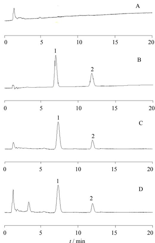
**Fig. 2** Representative chromatograms of blank plasma of dogs(A), blank plasma of dogs spiked with quercetin ( $0.1 \mu\text{g}\cdot\text{mL}^{-1}$ ) and IS (B), blank plasma of dogs spiked with hyperoside ( $0.1 \mu\text{g}\cdot\text{mL}^{-1}$ ) after pretreatment as described in paper (C), and plasma sample obtained 1 h after ig administration of hyperoside (D)
